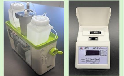
図6 e-HPLC(左)と光電比色計(右)
